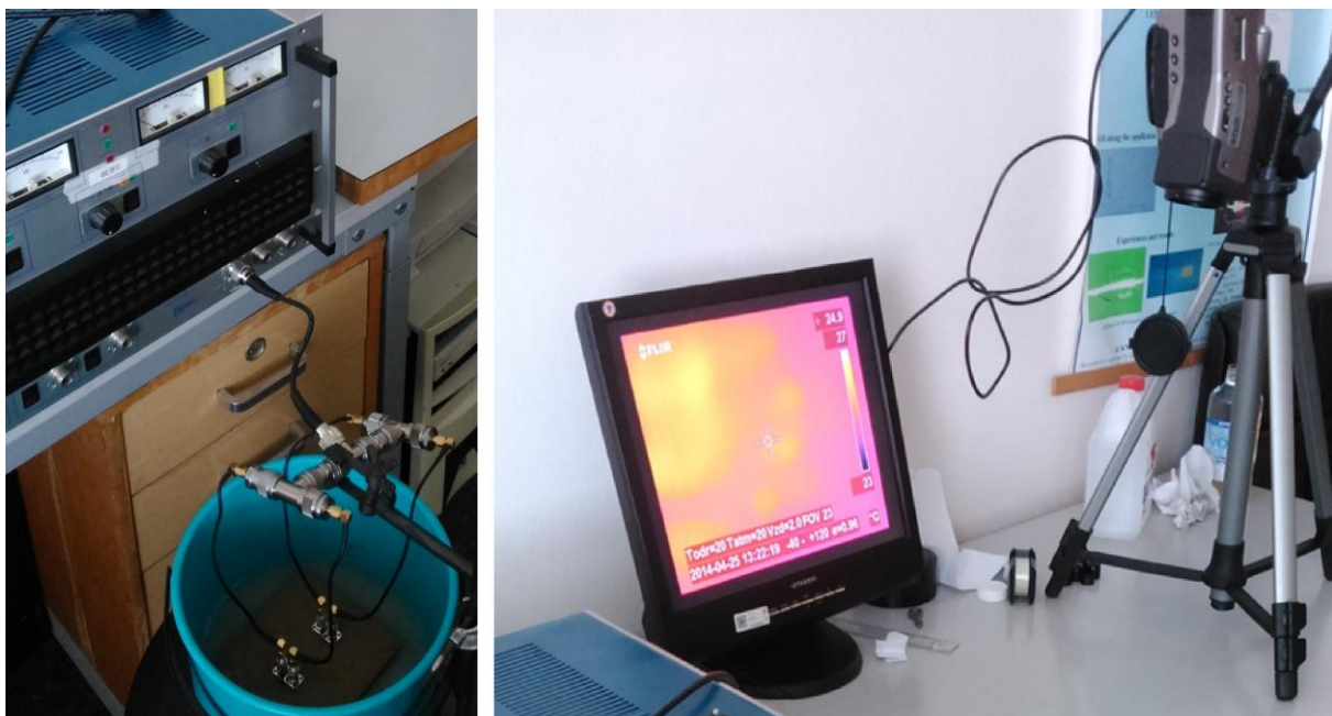
Picture 6-6 Measuring of the distribution of SAR into agar, (left) power generator with applicator, (right) thermal imager FLIR P25
